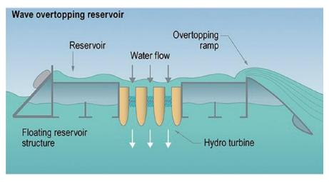
Figure 6: an example of wave energy technology: overtopping converters
